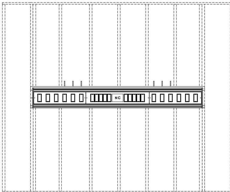
Add additional support members, as illustrated. Supports must be, at minimum, 20-gauge steel on 16" centerlines.
