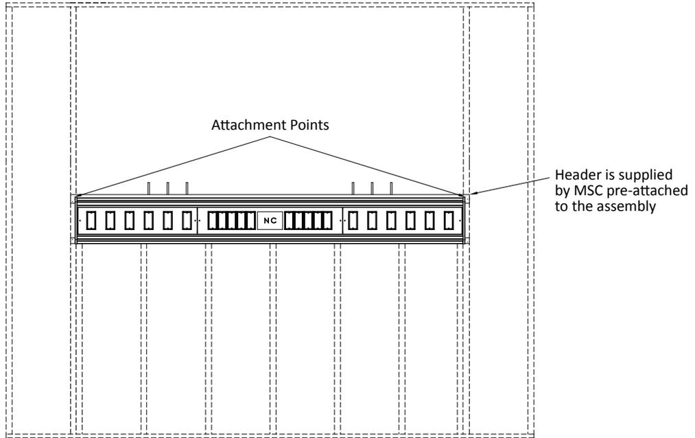
Place unit on footer and slide back into wall cavity. Attach unit with standard framing fasteners at locations indicated.
