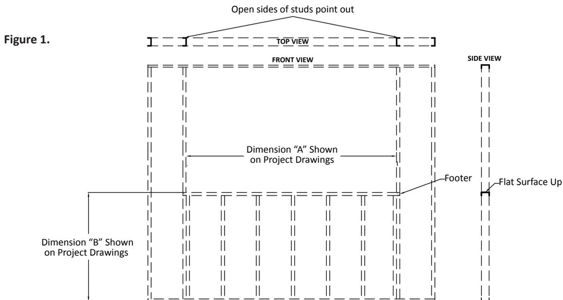
Frame opening as shown. Horizontal footer should be installed with opening in the down position. Stud wall must be, at minimum, 20-gauge steel studs on 16" centerlines.
